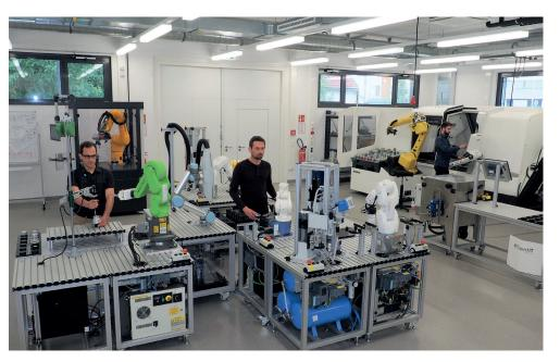
TU Graz smart factory is equipped with state-of-the-art machining, additive manufacturing centers and industrial robots from various manufacturers arranged in mobile, self-sufficient workstations.
