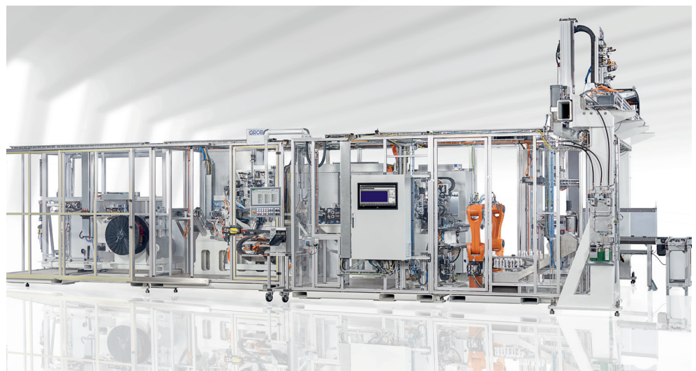
GROB is a leading manufacturer of machine tools and production plants for the automotive industry. The image shows a hairpin forming machine for electric motor production. (image courtesy of GROB)
