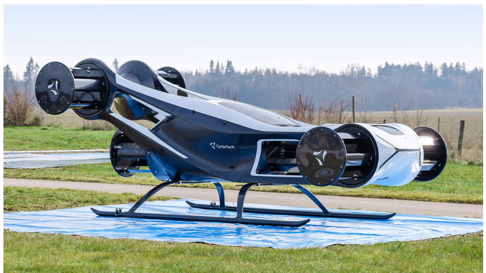
Six CycloRotors in two orientations give CycloTech's BlackBird technology demonstrator full spatial maneuverability, even in confined airspace and adverse weather conditions.
