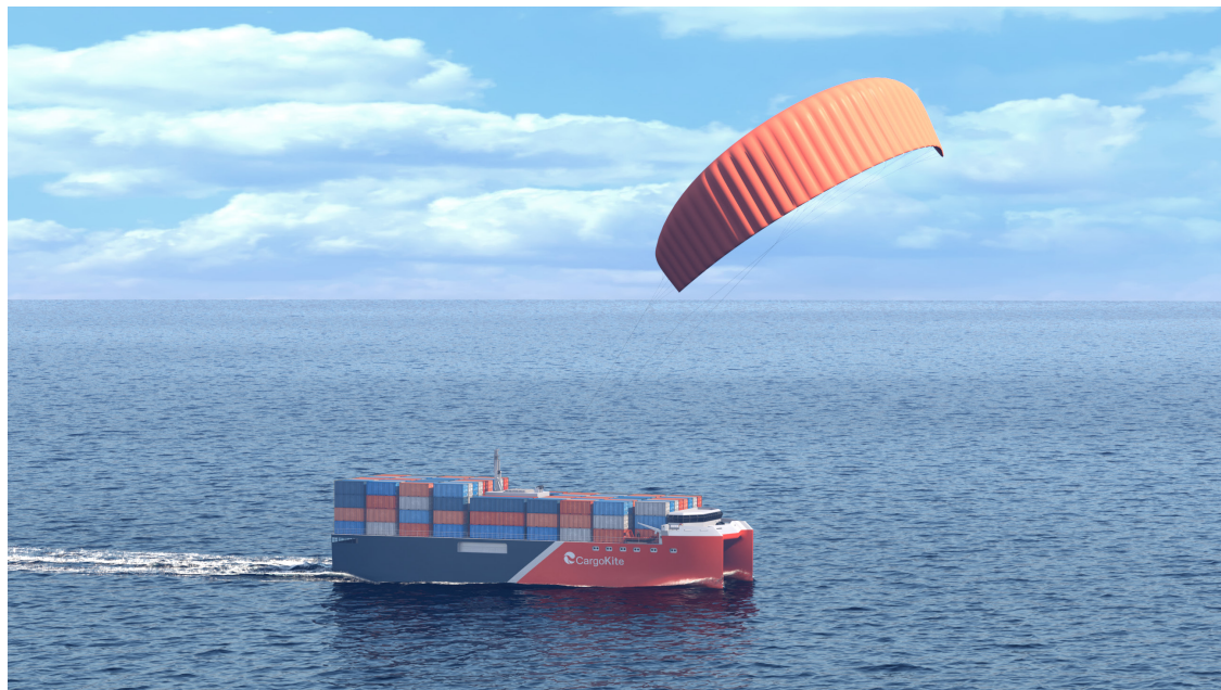
CargoKite uses a kite to develop a new kind of cargo sailing ship for the short sea and feeder market.
